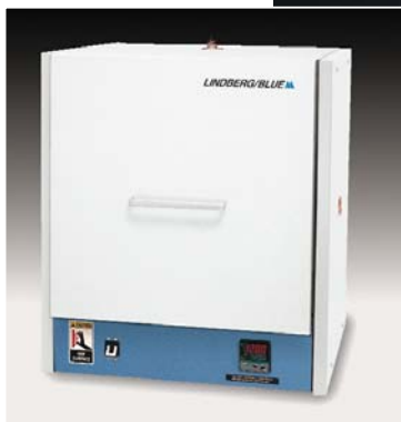
Model BF51842C 1200°C LGO Box Furnace with multiple segment, single program controller integrated into the main control panel. (below)
