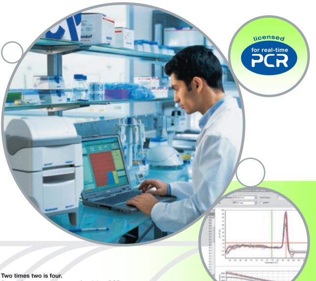
Depending upon your range of real-time PCR applications, select between two available detection systems - Mastercycler ep realplex2 and Mastercycler ep realplex4. Both are operated by the same realplex software, and both are equipped with an LED array to excite the fluorescent dyes in each individual PCR sample. The differences between each system include the number of fluorescence filters and photo-multipliers and the different, resulting levels of multiplexing capacity.
